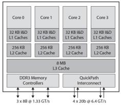
In the 1st Gen. Intel Core i7, each core had an L1 data cache and an L1 instruction cache, together with a unified L2 cache
