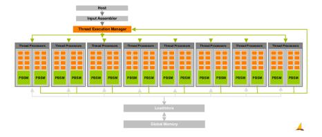
In a GPU, the small local memories have much smaller access time than the large shared memory.
