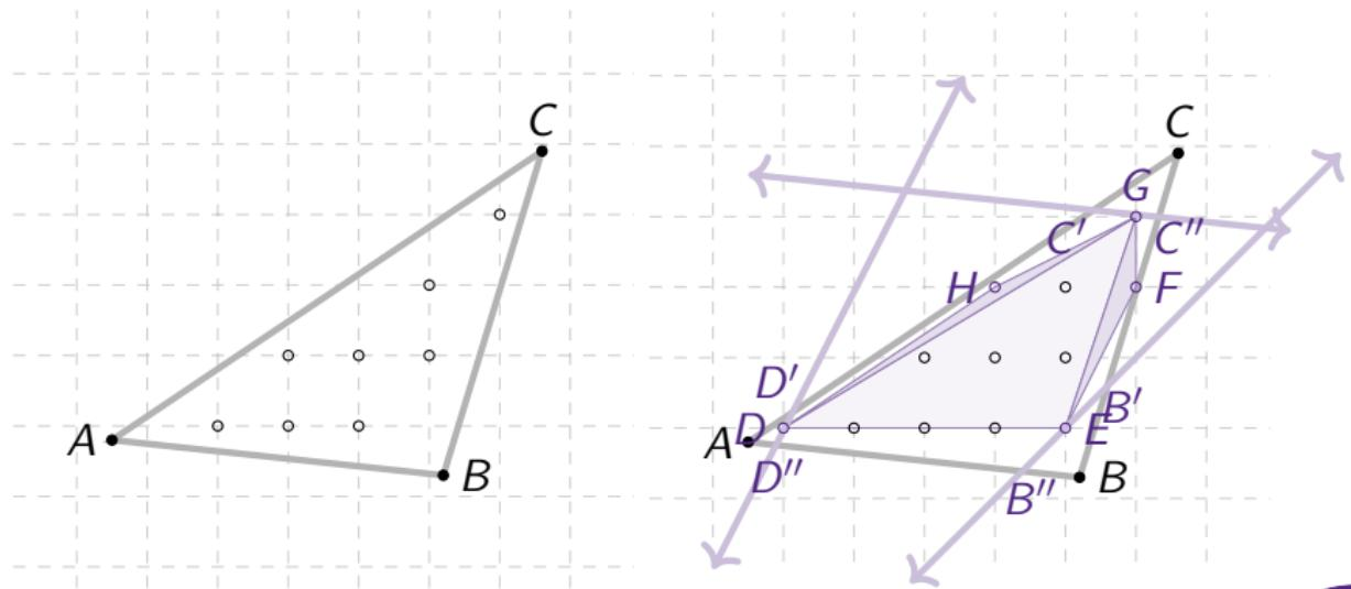
The **integer hull**  $\{D, E, F, G, H\}$  is formed by  $\{D, E, G\}$  and searching integer points  $\{F, H\}$  in quadrilaterals  $DD''B''E$ ,  $EB'C''G$  and  $D'DGC$ .
