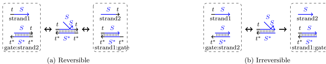
Figure 1: Example of basic DNA strand displacement reactions. Figure 1a is the reversible reaction \text{strand1} + \text{gate:strand2} \rightleftharpoons \text{strand1:gate} + \text{strand2} , and Figure 1b is the irreversible reaction \text{strand1} + \text{gate:strand2} \rightarrow \text{strand1:gate} + \text{strand2} . Each strand is represented as an arrow indicating 5'-to-3' orientation. t and S_1 are finite strings over \{A, C, G, T\} , and t^* and S^* are their 3'-to-5'-oriented Watson-Crick complements. The “toehold” region t is short enough (about 5 nucleotides) that it cannot provide sufficient binding strength to allow two strands to hybridize stably. Only if the longer (say, at least 15 nucleotides) “recognition” region S matches between strand1 and the base strand gate can strand1 displace strand2. Displacement occurs via an unbiased random walk but proceeds quickly compared to the time taken for strands to find each other in solution, so a successful displacement is modeled as occurring instantaneously upon binding of the toehold.
