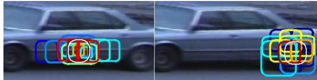
Figure 2: Patch Correlations. On each image, the patches most correlated with the white-circled patch are shown. Notice that in the left image, where the patch sits in an area with a highly visible horizontal structure, the most correlated patches all lie along the horizontal features. Contrast this with the right image, showing correlation of patches with a patch sitting on a wheel, where the most correlated patches are those that strictly overlap the white-circled patch.
