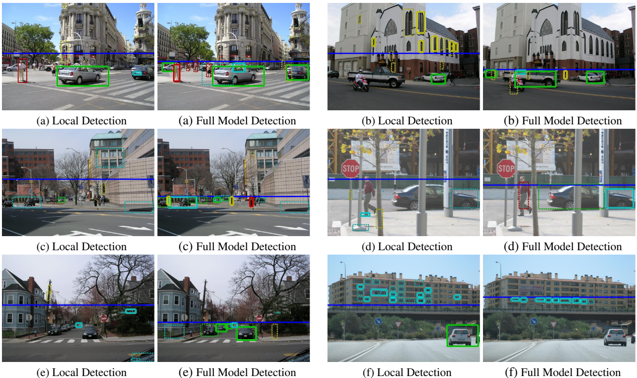
Figure 7. We show car and pedestrian results from our baseline local detector and after inference using our model. The blue line shows the horizon estimate (always 0.5 initially). The boxes show detection estimates (green=true car, cyan=false car, red=true ped, yellow=false ped), with the solid lines being high confidence detections (0.5 FP/Image) and the dotted lines being lower confidence detections (2 FP/Image). In most cases, the horizon line is correctly recovered, and the object detection improves considerably. In particular, boxes that make no sense from a geometric standpoint (e.g. wrong scale (d), above horizon (b), in the middle of the ground (e)) usually are removed and objects not initially detected are found. Of course, improvement is not guaranteed. Pedestrians are often hallucinated (c,e) in places where they could be (but are not). In (f), a bad geometry estimate and repeated false detections along the building windows causes the horizon estimate to become worse and the car to be missed.
